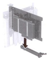
13 Insert the PCIe retainer into the computer ①, and then lower it ② into place.
