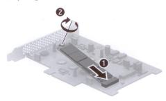
7 Insert the optional second M.2 module, label facing up, into the M.2 slot on the adapter at an angle ① and then secure the standoff to the adapter ②.
