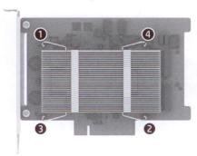
10 (HP Z8 only) Lift the PCle retainer by the access point 1, rotate it up 2, and then remove it from the computer 3.
