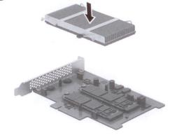
**9** Hold the middle of the heat sink down, and then press the hooks down in the following order.
