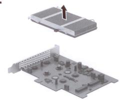
The protective covering over the thermal pads is perforated. If you are installing a single module, remove half. If you are installing both modules or a second module, be sure that the entire covering is removed.
