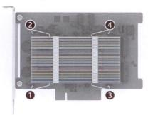
**7** Remove the heat sink from the adapter.
