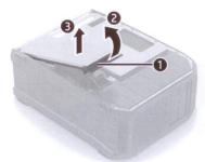
**11** Remove the PCIe slot cover.
