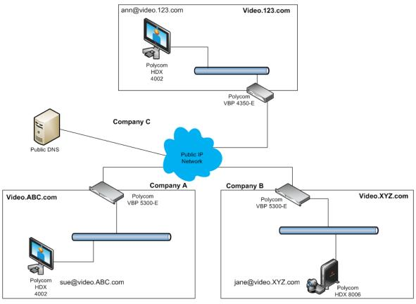
This example could also represent a single company that only had a single endpoint requirement and had no existing H.323 infrastructure. This diagram also shows the use of DNS-based ANNEX O (E.164@VBP-WAN-IP) dialing, and again direct gatekeeper neighboring is also possible by configuring prefix based gatekeeper neighboring.
