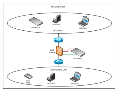
This Polycom VBP installed in a DMZ configuration will also need to pass all of the video traffic through the firewall. The same concerns apply to this design as described earlier in *Polycom VBP Operating Outside NAT Firewall* on page 9 design. The implementation is can be done with the WAN port of the VBP in a
