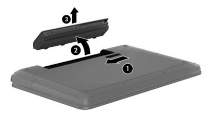
Reverse this procedure to install the battery.
