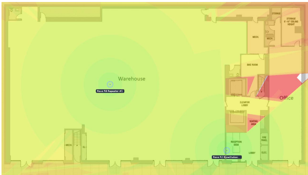
Floor plan example with one Rove B2 base station and one paired Rove R8 repeater
